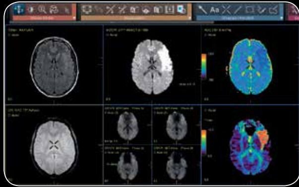
Figure 3B. Integrated Registration is used to retrospectively co-register the DWI and FGRE T2* to the T2 FLAIR. Motion correction option in BrainStat AIF is selected to realign all phases of the DSC scan. Notice the recovered shape of the brain anatomy on the Tmax map.
